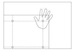
Press panel onto SpinFix clips to mark the fixing points.
