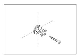
Fix SpinFix button and washer to substrate.
